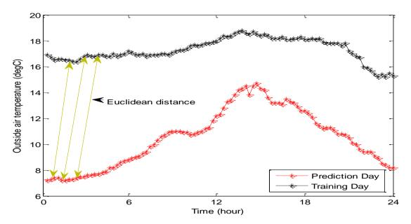
Fig. 3: DTW illustration of outside air temperature
