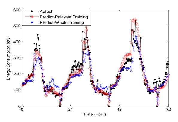
Fig. 6: Prediction of heating energy consumption for working days
