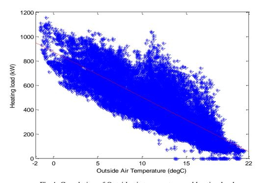
Fig.4: Correlation of Outside air temperature and heating load
