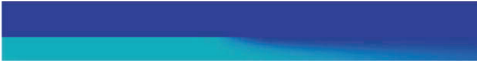
Figure 18 (b) Concentration field when x_F = 160W , for \Delta = 0.5 and Pe = 10 in the incompressible flow.
