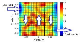
Fig. 5 Current density distribution (A cm<sup>-2</sup>) recorded by the S++
