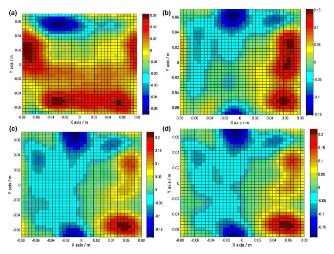
Fig. 9 Reconstructed current density change from magnetic field measurement for air stoichiometry ranging from 2 to 2.2 (a), 3 (b), 4 (c) and 4.5 (d)
