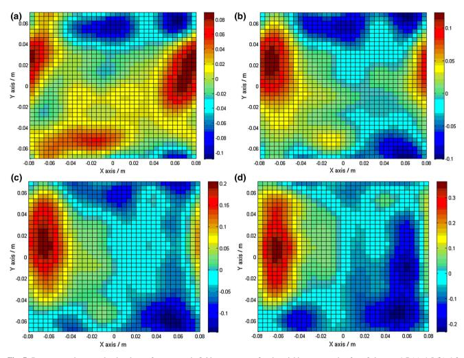
Fig. 7 Reconstructed current density change from magnetic field measurement for air stoichiometry ranging from 2 down to 1.7 (a), 1.5 (b), 1.3 (c) and 1.15 (d)
