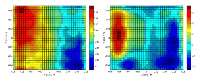
Fig. 8 Current density changes (A cm $^{-2}$ ) from S++ card (*left*) and reconstructed current density change from magnetic field measurement (*right*) for air stoichiometry ranging from 2 down to 1.15
