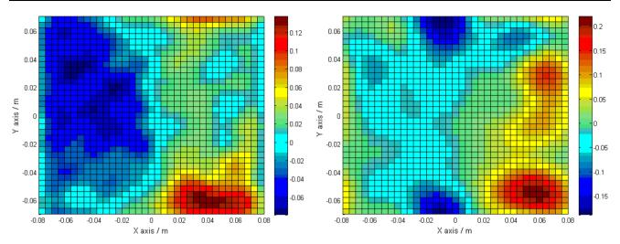
Fig. 10 Current density changes (A cm $^{-2}$ ) from S++ card (left) and reconstructed current density change from magnetic field measurement (right) for air stoichiometry ranging from 2 to 4.5
