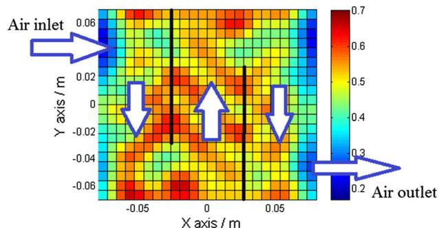
Fig. 5 Current density distribution (A cm<sup>-2</sup>) recorded by the S++ card
