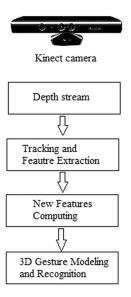
Figure 1: Flowchart of the proposed 3D dynamic gesture recognition technique.
