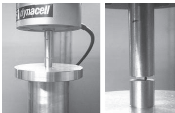
Figure 1 Side crushing strength test of a cylindrical support.
