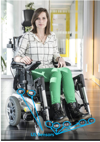
Fig. 4. Robotized wheelchair equipped with ultrasound sensors located on the side and on the rear of the body, as well as in footplates.
