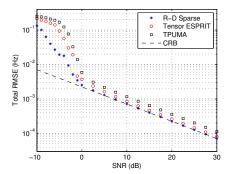
Figure 7: Frequency total root-mean square error for a 3-D signal containing 3 modes with identical modes in two dimensions (Signal #3), with close modes in the first dimension (0.28,0.12,0.2).  $(M_1,M_2,M_3)=(10,10,10)$ . 200 Monte-Carlo.
