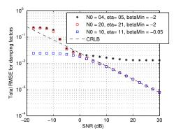
Figure 4: Damping factor RMSE using R-D sparse algorithm with different  $\eta_{\alpha}$ ,  $\beta_{\min}$  and N(0). 2-D signal containing a single tone (Signal #1).  $(M_1, M_2) = (10, 10)$ . 1000 Monte-Carlo trials.
