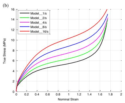
behaviour is the beginning of the stress–strain curve (when the strain is lower than 0.3): the experimental data initial slope seems to increase when the strain rate rises. This is in contradiction with the results of the model.
