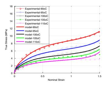
**Fig. 6** The data experimental (the points) and the results of the viscoelastic model (the lines) at 8 s<sup>-1</sup> under different temperatures (90 °C,95 °C,100 °C,105 °C,110 °C)
