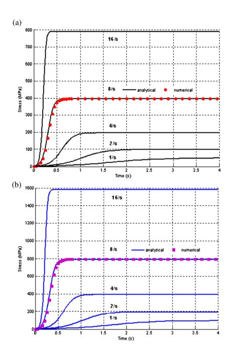
equibiaxial test. Equation 17 gives the  $\eta_0 h$  evolution versus the equivalent viscous strain  $\overline{\varepsilon}_{\nu}$  for each strain rate condition. The equibiaxial tests have been carried out for five global strain rates (1 s<sup>-1</sup>, 2 s<sup>-1</sup>, 4 s<sup>-1</sup>, 8 s<sup>-1</sup>, 16 s<sup>-1</sup>).
