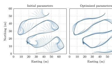
Figure 8: Left: Model errors for different sets of parameters. Leica refers to the theodolite ground truth measurements. Middle: Ground truth trajectory (black) and model trajectories (blue) over 20 s for the initial parameters. Right: trajectories after optimization.
