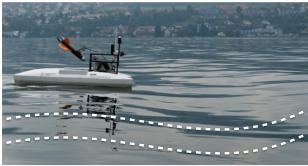
Figure 1: State estimation needs on a lake at different scales. *Top*: Overview of Lake Zurich, for which 2D state estimation fulfills the needs of most application cases. *Bottom*: Zoom on the ASV Lizhbeth with low frequency waves requiring 3D state estimation to observe small scale features.
