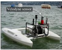
Figure 4: *Left:* The reflective pole used to assess the distortion of point clouds. *Right:* The temporarily mounted Velodyne sensor on the ASV.
