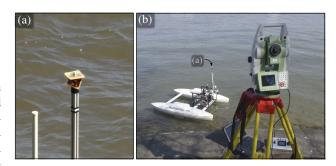
Figure 3: Material used for position ground truth. (a) Specialized prism used as target for automatic tracking. (b) A theodolite (Leica Total Station TS15) mounted on shore and tracking the ASV.
