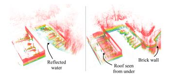
Figure 13: Comparison of a professional land survey unit and a low cost laser rangefinder mounted on a mobile platform. The area used for the experiment is a boathouse where the ASV is usually stored. *Left*: An assembly of 5 scans taken with a Leica MS50 on Sept. 3, 2014. *Right*: Reconstruction based on all points acquired from the robot Lizhbeth. Colors represent the elevation, red being high and blue being low.
