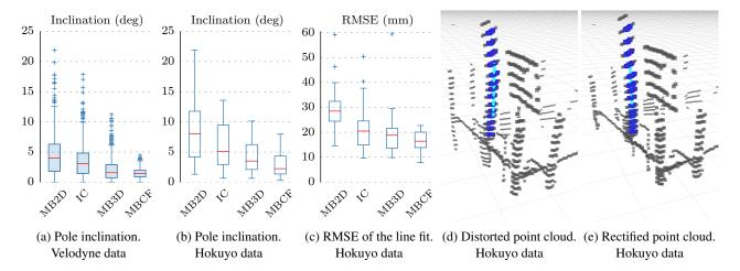
Figure 11: Results of the *pole experiments*. The resulting inclinations of the pole in the Velodyne data set are depicted in (a). The results of the line fitting for the Hokuyo data is shown in (c) and (b). An example of a point cloud (dark grey) with the extracted points on the pole (blue) and the fitted line (cyan) is shown in (d) and (e).
