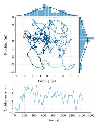
Figure 15: GPS noise analysis of a stationary point (on the shore) over 24 minutes. *Top*: 2D error of the GPS coordinates with respect to the mean. The coloring of the points corresponds to the temporal evolution. A fitted Gaussian distribution is overlaid onto the error histograms. *Bottom*: Evolution of the northing error through time.
