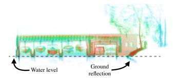
Figure 16: Front view of the boathouse. The dashed line represents the approximate position of the water level. The color of the point represents the laser intensity, red being high and blue low.
