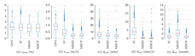
Figure 10: Results of the position evaluation based on theodolite ground truth. The metrics are: position error  $(e_{pos})$ , velocity error  $(e_{vel})$ , position discontinuity  $(d_{pos})$ , velocity discontinuity  $(d_{vel})$ , attitude discontinuity  $(d_{att})$ . For the first two panels, the raw GPS data is shown as a baseline.
