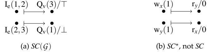
Figure 2: A sequential history for an instance of \mathcal{G} and a cache consistent history for an instance of \mathcal{M}_{\{x,y\}} that is not sequentially consistent
