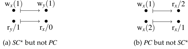
Figure 5: These histories on \mathcal{M}_{x,y} show that PC is not comparable with SC^*
