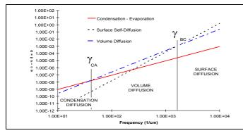
Fig. 1. Values of the exponential terms of decay coefficient of each diffusion component  $B\omega^{4n}$ ,  $C\omega^{3n}$  et  $A\omega^{2n}$  for different frequencies value  $\gamma$  with  $\gamma=\lambda^{-1}$ . Applied on the aluminum sheet annealed at 550°C, one gets  $A=2.3\,10^{-13}\,CGS$ ,  $B=10^{-19}\,CGS$ ,  $C=10^{-15}\,CGS$ .
