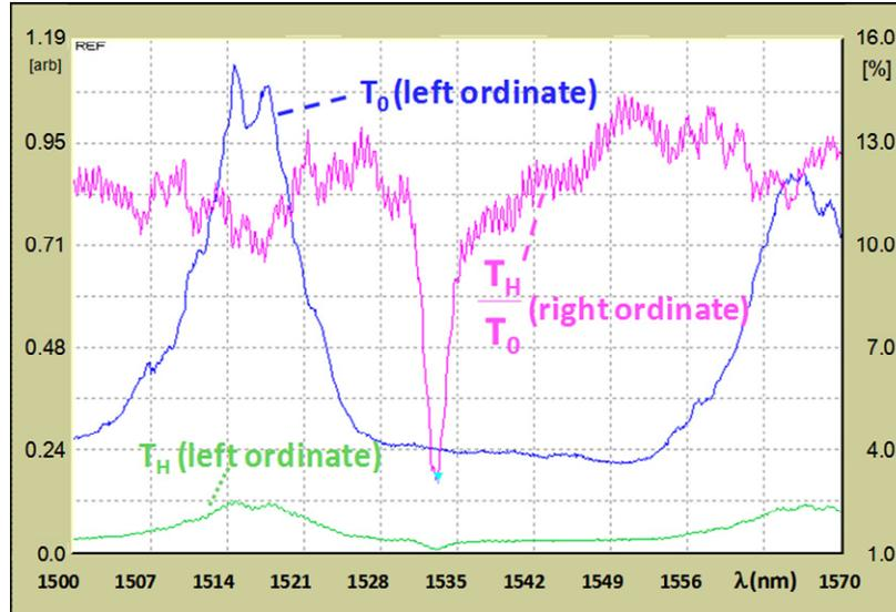
Fig. 7. Wavelength scan in the C-band of the transmission under normal incidence and linear polarization of one of the 31 mirrors fitting the specifications ( $T_0$ : transmission in region without the hexagonal grating,  $T_H$ : transmission with hexagonal grating)
