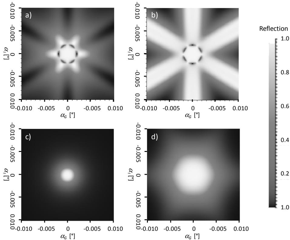
Fig. 3. 2D angular spectra of the reflection from a slab waveguide with hexagonal set of holes designed for a disc laser mirror sketched in Fig. 9 upon excitation of the only propagating  $TE_0$  mode: a) TE incident polarized and b) TM polarized excitation by a double-sided corrugation, c) TE and d) TM excitation by a single-sided corrugation.
