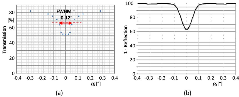
Fig. 15. Angular scan of the transmission of a resonant submirror for linearly polarized incidence. (a) Measured transmission for a spectrometer resolution of 0.5 nm and a beam divergence of  $0.06^\circ$ , not corrected for backside reflection. (b) Simulation of the transmission taking into account the spectrometer resolution and beam divergence from the experiment, without backside reflection.
