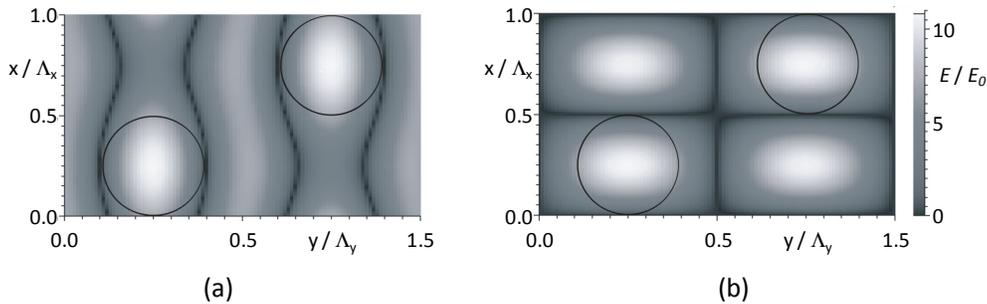
Fig. 10.  $\text{TE}_0$  modal electric field modulus distribution over one period in the  $\text{Si}_3\text{N}_4$  waveguide of the element of Fig. 9 at resonance under normal incidence of a x-polarized wave. The black circles indicate the position of the holes at the upper surface of the cover layer. (a) Modulus of the x component of the electric field, (b) of its y component.
