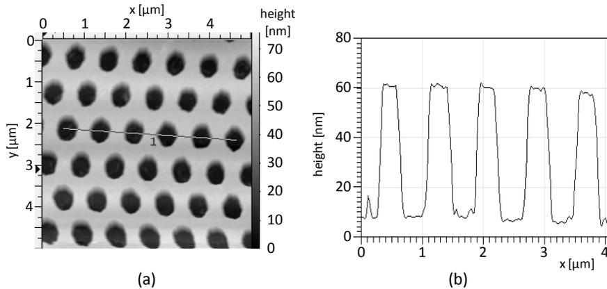
Fig. 12. (a) 2D AFM scan of the set of holes of Fig. 11 after wet etching into the SiO<sub>2</sub> cover layer, (b) 1D profile scan of a) showing the grating height.
