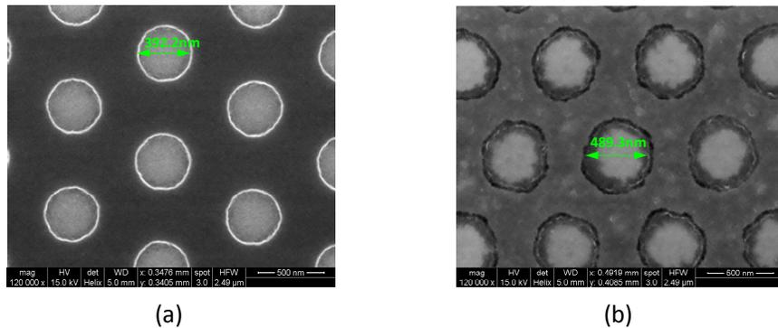
Fig. 11. (a) SEM image of a set of developed holes of 816 nm period in a ~120 nm thick photoresist layer, (b) same set of holes after wet etching into the SiO<sub>2</sub> layer.
