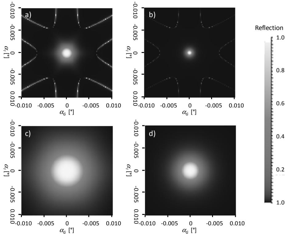
Fig. 4. 2D angular spectrum of the reflection from an hexagonal set of holes of the back-mirror sketched in Fig. 5 designed for a microchip laser with  $TM_0$  mode excitation. Curves a) and b): TE and TM incident polarization onto a multilayer system where all interfaces have conformal undulation. Curves c) and d): TE and TM incident polarization with single-sided undulation of the upper waveguide boundary.
