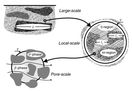
Fig. 1. The three scales of the problem: the pore-scale composed of a solid phase ( $\sigma$ ) and a fluid phase ( $\beta$ ); the local-scale consists of two embedded homogeneous regions ( $\eta$  and  $\omega$ ); the large-scale that still presents some macroscopic heterogeneities.
