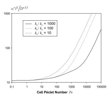
Fig. 8. Large-scale mass transfer coefficient as a function of the cell Péclet number for different permeability ratios.
