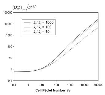
Fig. 7. Large-scale longitudinal dispersion coefficient in the  $\eta$ -region as a function of the cell Péclet number for different permeability ratios.
