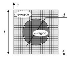
Fig. 3. Two-dimensional nodular unit cell.
