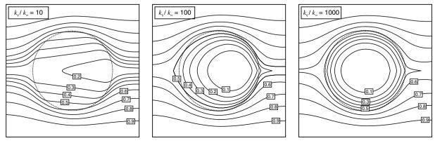
Fig. 6. Isoconcentrations in the 10th nodules at  $t = 4 \times 10^4$  s for different permeability ratios.
