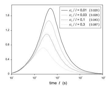
Fig. 15. Evolution of the non-equilibrium criterion as a function of time in a nodular system for different local-scale dispersivities. The Damköhler is given between brackets for indication.
