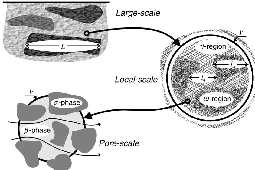
Fig. 1. The three scales of the problem: the pore-scale composed of a solid phase ( $\sigma$ ) and a fluid phase ( $\beta$ ); the local-scale consists of two embedded homogeneous regions ( $\eta$  and  $\omega$ ); the large-scale that still presents some macroscopic heterogeneities.
