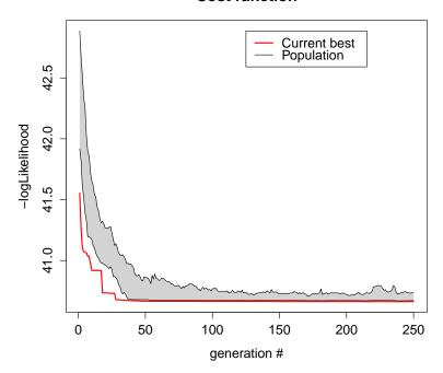
Figure 6: Evolution of the value of the fitness function of the current best solution (bold red line) and of the current population (the grey area shows the interval between the 10th and 90th percentile). Most of the cost function improvement is achieved after 30 generations. The population evolves towards small function values only but do not converge towards a unique value.
