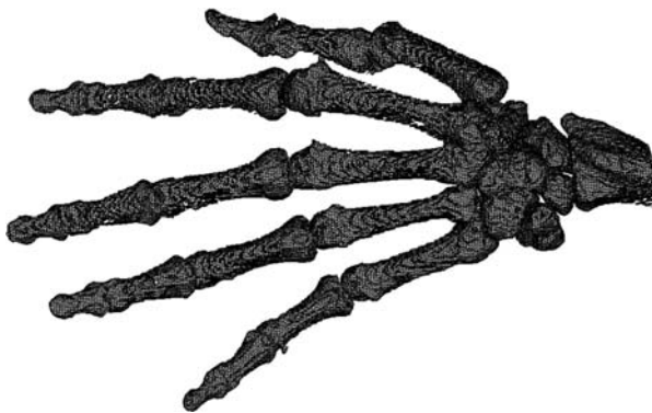
Figure 3. STL meshing of the hand with tria before the reconstruction of the surfaces.
