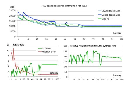
Figure 5: Exploration of an IDCT coprocessor in order to compare our HLS-based estimation with logic synthesis. Comparisons of slice estimations are shown on the top curve and the bottom ones show the accuracy of the estimation and the speedup over logic synthesis.
