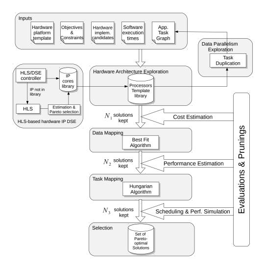
Figure 7: Flow of the Design Space Exploration.
