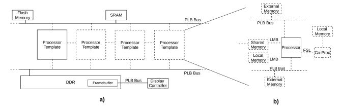
Figure 2: A graphical representation of an architecture template and a detailed view of the processor template. Solid lines indicate fixed parts (level 1) of the architecture while dotted lines represent potential instantiations (levels 2 and 3) that are decided during DSE.
