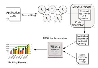
Figure 6: Flow of the on-target profiling step.
