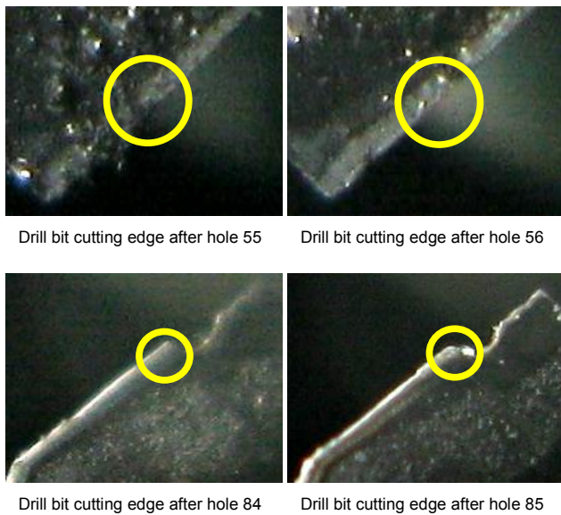
Figure 6: Pictures of the drill bit taken after 55, 56, 84 and 85 holes. AE signals that are remarkable after performing AE count rate (holes 56 & 85) correspond to drill bit cutting edges chipping
