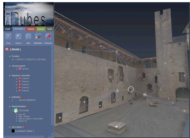
Figure 5. Semantic qualification of a 3D representation in Nubes Visum. The user can select a morphological entity, assign a vocabulary term, choose a type of representation (point cloud, profiles, polygons, etc.), qualify entities by custom attributes and create related reference marks.
