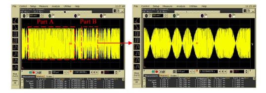
Fig.8: Time measurements for communication between reader /tag.
