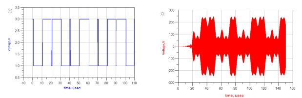
Fig3: Digitaldata to be transmittedFig4: Carrier modulated bythedata
