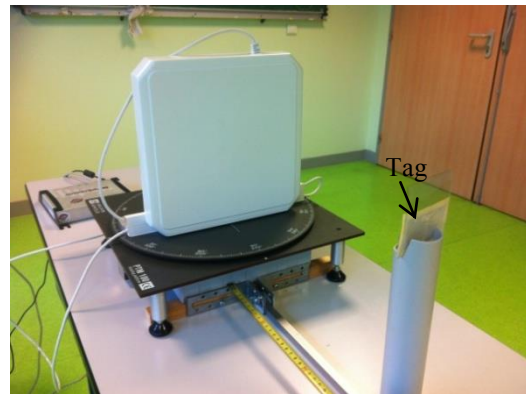
Fig.7.b: Tag mounted on the sliding support
