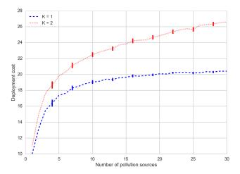
Fig. 4: Deployment cost average and the 98% confidence intervals depending on the number of pollution sources. A 400mX1000m area is considered, nodes are placed at a height of 20m and a sink is considered ten times much expensive than a sensor.
