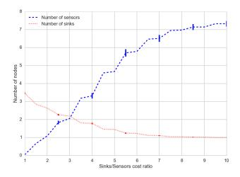
Fig. 3: Number of sinks and sensors average and the 98% confidence intervals depending on their cost ratio in the case of 1-Coverage. A 400mX1000m area is considered and 5 pollution sources are randomly generated. Nodes are placed at a height of 20m.
