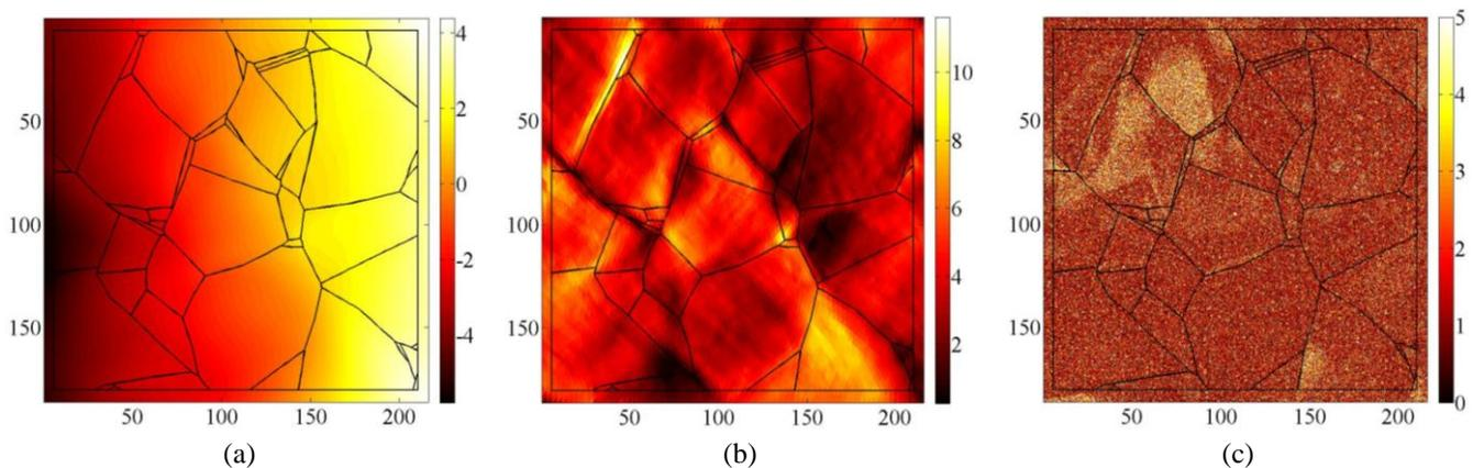
**Fig. 2:** Displacement field expressed in micrometers (a) and strain field in percents (b) along the horizontal loading direction measured by DIC for a macroscopic strain of 5%. Corresponding correlation residuals expressed in percentage of the picture dynamic range (c). The axes are in micrometers. The microstructure boundaries are shown as black lines
