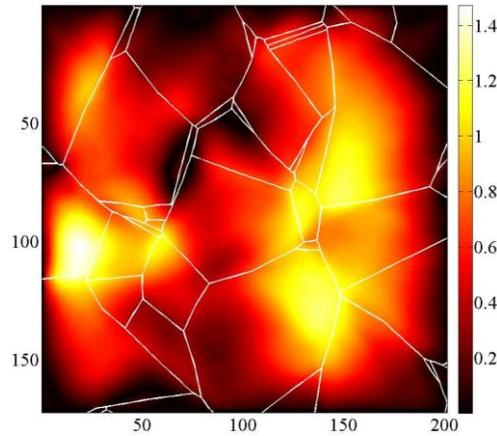
**Fig. 3:** Absolute value of the difference between measured and simulated displacement fields along the horizontal direction for a macroscopic strain of 5 %. The field and the axes are expressed in micrometers. The microstructure boundaries are shown as white lines
