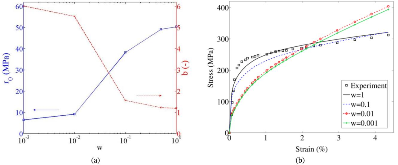
**Fig. 4:** Values of the identified parameters  $r_0$  and  $b$  as functions of  $w$  (a). Stress-strain curves obtained by homogenization at convergence of the identification performed with different values of  $w$ , compared to the experimental curve (b)
