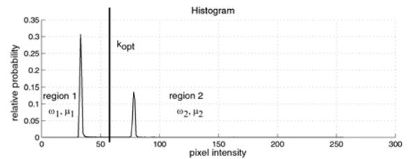
Fig. 6. Histogram and parameter for Otsu's method.
