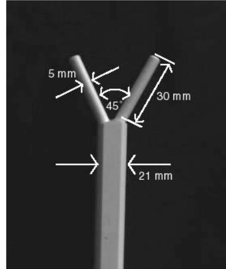
Fig. 3. Instrument made of PVC.
