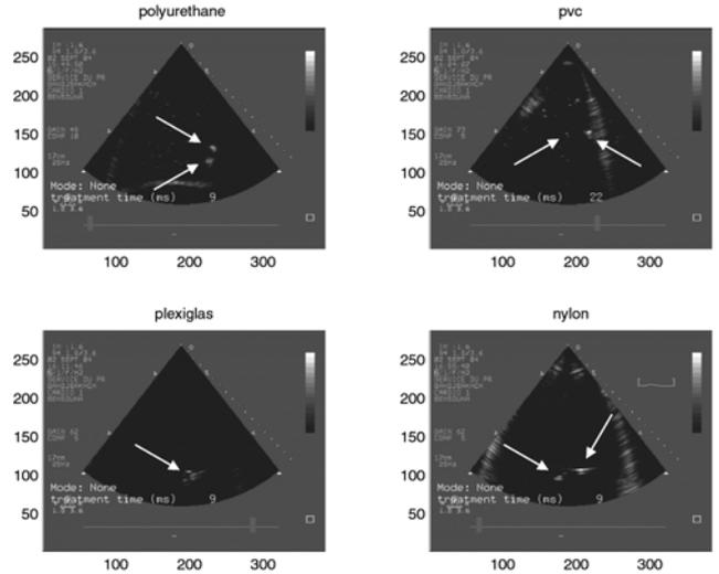
Fig. 8. Instrument echoes for materials used.
