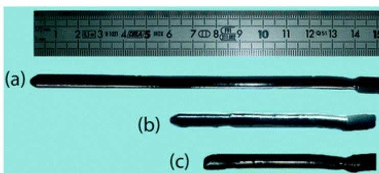
Fig. 2 Typical examples of as-grown single crystals of (a)  $\text{Pr}_2\text{NiO}_{4+\delta}$ ; (b)  $\text{Pr}_{1.9}\text{Sr}_{0.1}\text{NiO}_{4+\delta}$  and (c)  $\text{Pr}_{1.5}\text{Sr}_{0.5}\text{NiO}_{4+\delta}$  obtained by the floating zone method under oxygen flow.
