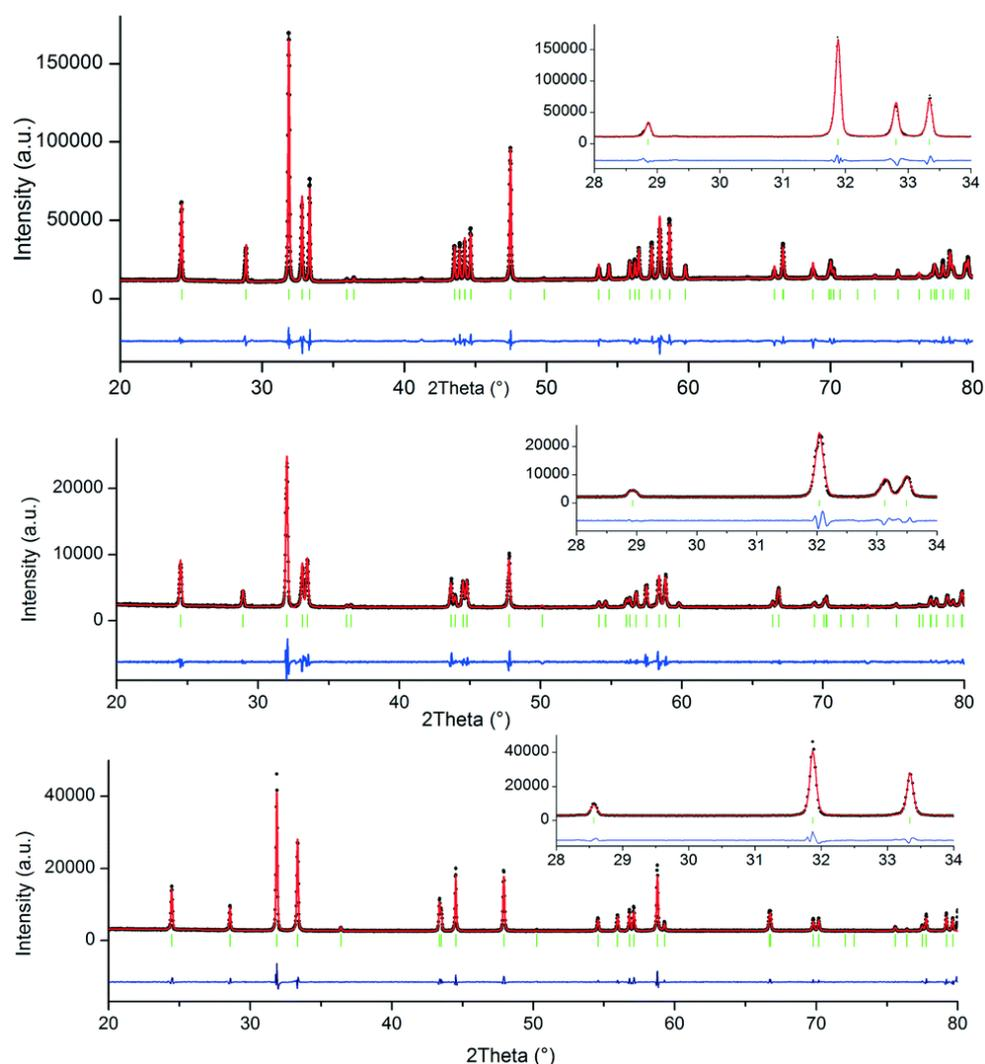
Fig. 3 X-ray diffraction patterns of crushed NSNO single crystals after annealing at 430 °C. The upper diagram was obtained for  $x = 0.00$ , the middle for  $x = 0.1$  (both orthorhombic), while the bottom corresponds to  $x = 0.5$  with tetragonal symmetry. We underline the excellent crystalline quality of all compounds, showing FWHM close to the resolution function of the diffractometer. Similar patterns have been obtained for PSNO crystals (Fig. S2† in the ESI).
