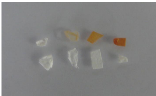
Figure 5. The image (from left to right) of PCL 80 , f-PCL-N 3 -20, f-PCL-N 3 -40 and f-PCL-N 3 -60 fibers after incubation with FITC-alkyne, with (top line) and without catalysts (bottom line), demonstrates successful attachment of the FITC fluorophore by click chemistry and macroscopically visible differences in the grafting ratio
