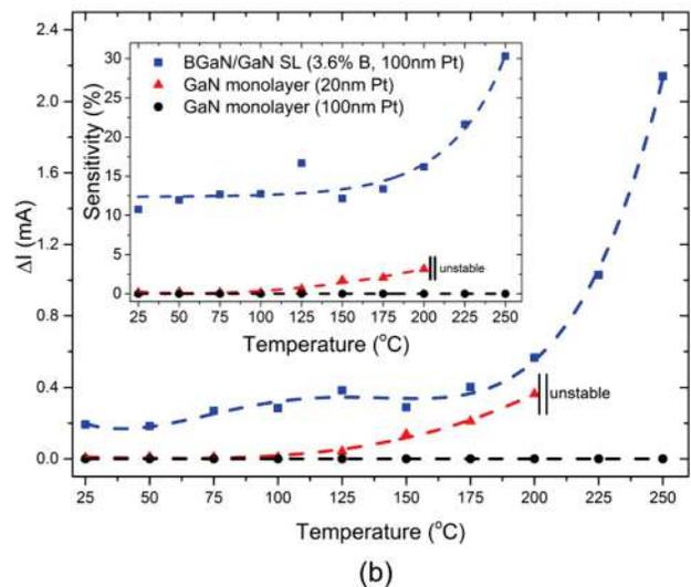
FIG. 1. (a) Sensor device and (b) comparison of the temperature dependence of  $\Delta I$  and S (inset) of BGaN/GaN SL and GaN sensors to 450 ppm NO<sub>2</sub> at 5 V bias.
