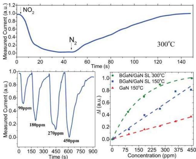
FIG. 3. Measured current (in arbitrary units) for the BGaN/GaN SL sensors under intermittent flows of 450 ppm  $\text{NO}_2$  and pure  $\text{N}_2$  gas at  $300^\circ\text{C}$  and 5 V bias (top), repeated between 90 and 450 ppm  $\text{NO}_2$  (bottom left), and  $\Delta I$  as a function of concentration for various temperatures, showing a linear response below  $300^\circ\text{C}$  (bottom right).
