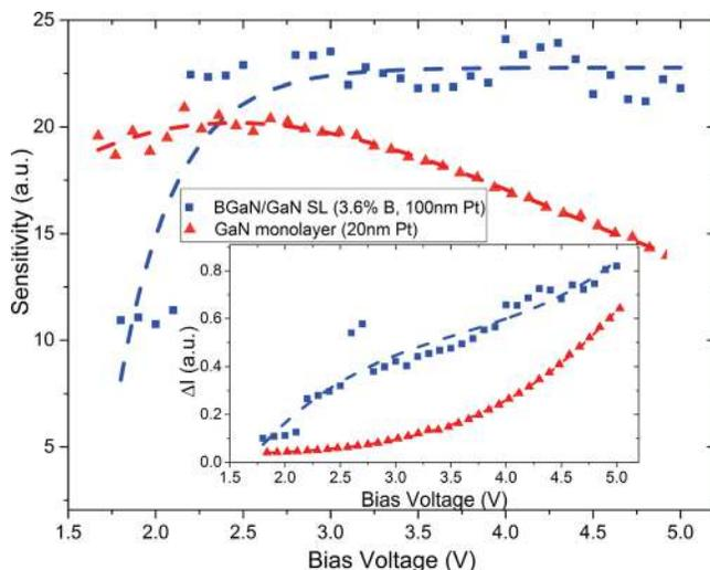
FIG. 2.  $\Delta I$  and  $S$  of the BGaN/GaN SL and GaN sensors in 450 ppm  $\text{NO}_2$  as a function of applied bias at  $150^\circ\text{C}$ . Values are given in arbitrary units so that the trends can be placed on the same scale.
