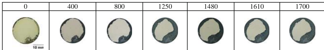
Fig. 3 Pictures of the SPS MCNG-2+Cu system versus the number of cycles at 1,100 °C
