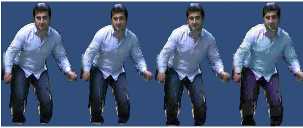
Figure 4: From left to right: Uncompressed, low compression, medium compression, high compression
