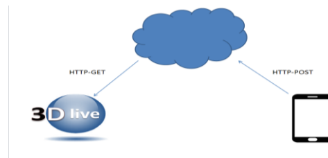
Fig. 7: Android application connection to 3DLive system through webservice.
