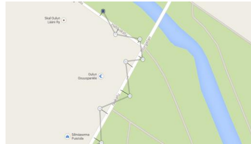
Fig. 6: Path of the GPS location updates with closest-to-road vectors.
