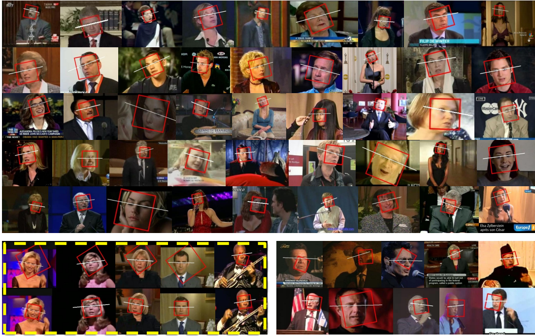
Fig. 10 Good (first five row) and problematic (last two row) estimations from YouTube C dataset where the white line presents the ground-truth orientation. Some of the problematic examples (e.g., first five column of the last two row highlighted by the yellow rectangle) are singular incidents and they are corrected in the following frames. The problem occurs when the frontal face detector in Level 1 detects a large false positive face which actually includes a real face. The errors from these examples also used in MAE computation
