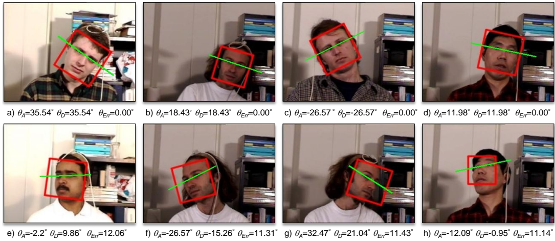
Fig. 12 Examples of the best (first row) and worst (second row) results obtained from BUFT dataset. Oriented rectangles in red color presents our face detection result with the corresponding orientation while the green lines shows the ground-truth orientation
