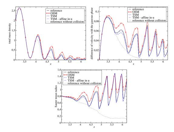
Figure 11: Results for the nozzle test case with OSM and affine TSM with a constant or an affine reconstruction of the velocity in the section: total mass density (top left), mean velocity minus gas velocity (top right), Sauter mean radius (bottom).
