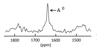
**Figure 4.** Detailed region of the 1D quantitative spectrum for the 85 nm thick coating grown at 480 °C
