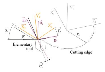
Figure 8: Local geometry of the insert.
