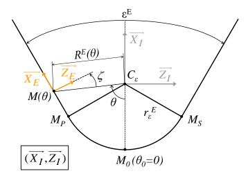
Figure 7: Polar parameterisation of the cutting edge.
