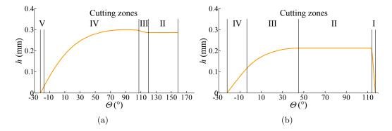
Figure 11: Uncut chip thickness along the active cutting edge: (a) DCMT11T304 + SDHCL; (b) SCMT120404 + SSDCL.
