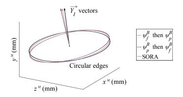
Figure 6: Comparison between SORA method and two matrix compositions: calculated circular cutting edges ( $r_{\varepsilon} = 3 \text{ mm}$ ) in  $\mathcal{R}_{Machine}$  for  $\psi_f^B = \psi_p^B = -30^{\circ}$ .
