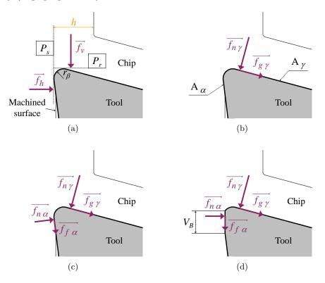
Figure 1: Possible applications of the local forces: (a) in the  $(\vec{o}, \vec{v}, \vec{h})$  basis; (b) on the rake face; (c) on the rake and clearance faces; (d) on the worn clearance surface (or the rounded edge).
