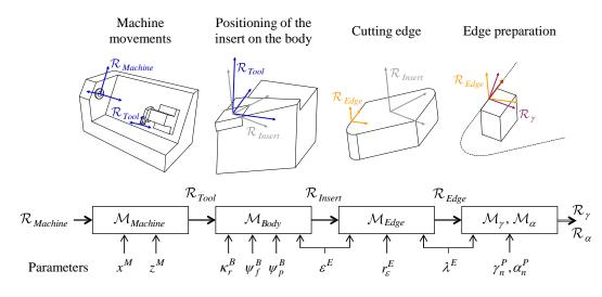
Figure 3: Graphic summary of the method, illustrated for turning.
