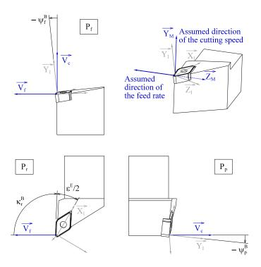
Figure 5: Positioning of the insert on the tool body: cutting edge angle  $\kappa_r^B$  and tilting angles  $\psi_t^B$  and  $\psi_n^B$  (see also [36]).
