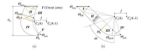
Figure 10: Cutting zones for cylindrical turning with a rhombic insert, for two cases: (a)  $\kappa_r > 90^\circ$   $(a_p > a_{p \, lim}$  and  $f > f_{lim})$ ; (b)  $\kappa_r < 90^\circ$   $(a_p > a_{p \, lim}$  but  $f < f_{lim})$ .
