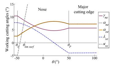
Figure 12: Calculated working cutting angles along the active cutting edge.
