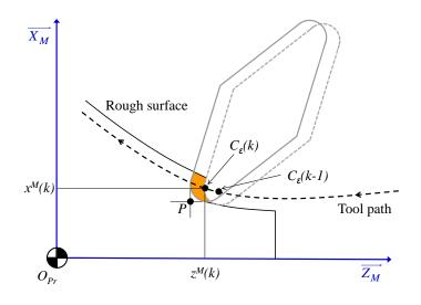
Figure 4: Machine axis and tool trajectory.
