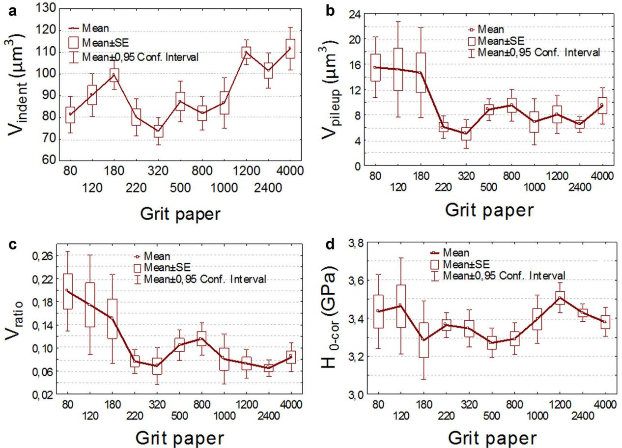
Fig 16. Histogram of (a) the indentation volume  $V_{\text{indent}}$ , (b) pile-up volume  $V_{\text{pileup}}$ , (c)  $v_{\text{ratio}}$ , and (d) modified hardness  $H_{0\text{-cor}}$  versus different polishing grit paper.
