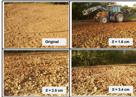
Fig. 3 Experimental set up of different surface roughness (described by RMS height s ) over bare soils.
