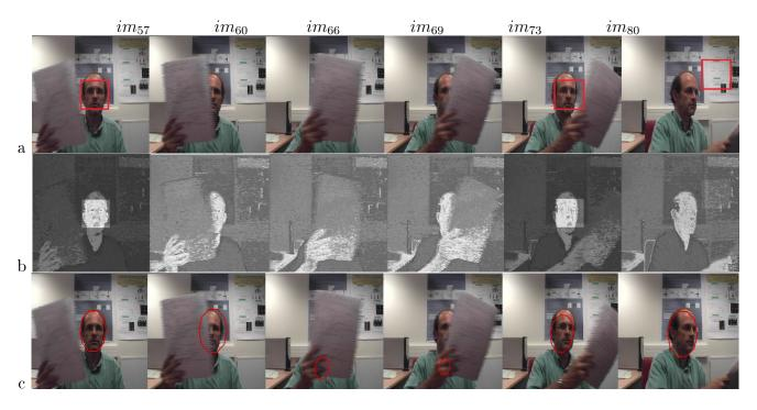
Figure 12: Face tracking for sequence #1: a) Bounding box supplied by the VJ face detector; b) Pignistic probability of the face model; c) Ellipse resulting from particle filter.
