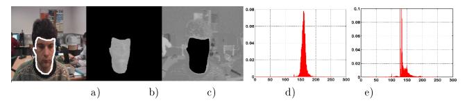
Figure 6: Initialization on sequence #2: a) selected area of the face on the first image of the video; b) source  $s_1$ : face zone; c) source  $s_1$ : background; d) distribution  $P(s_1|H_1)$ ; e) distribution  $P(s_1|H_2)$ .
