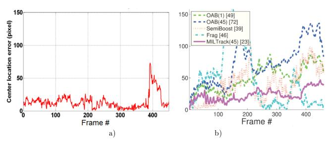
Figure 14: Tracking results (center location error) on David Indoor sequence, with: a) the proposed method; b) various algorithms according to Babenko [33].
