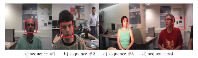
Figure 5: Rectanguler bounding box BB produced by the VJ face detector in various sequences: a), b), c) correct detections; d) false detection.
