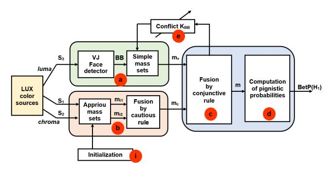
Figure 3: Block-diagram of the evidential face model: a) mass sets of the VJ face detector; b) color mass sets; c) fusion of VJ and color mass sets; d) computation of pignistic probabilities in the TBM; e) conflict management feedback; i) initialization.
