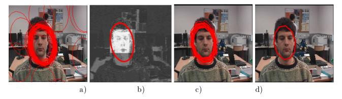
Figure 10: Sequence #2: a) particles generated for the center estimation stage (N = 50); b) best position result; c) particles generated for the size and pose estimation step; d) final best ellipse in size and pose.
