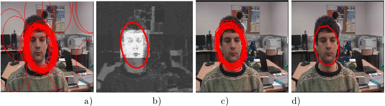
Figure 10: Sequence #2: a) particles generated for the center estimation stage ( $N = 50$ ); b) best position result; c) particles generated for the size and pose estimation step; d) final best ellipse in size and pose.
