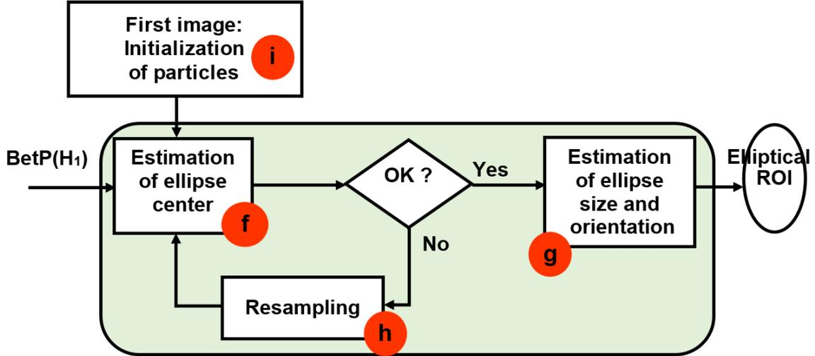
Figure 9: Block-diagram of the tracking algorithm by particle filtering.
