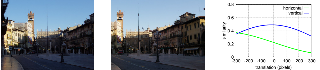
Figure 6: Matching example of two images and similarity estimation for all possible image translations. Image on the left undergoes translation independently to the horizontal and the vertical direction. Modulated VLAD is used for the example.
