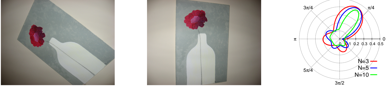
Figure 4: Matching example of two images and similarity estimation for all possible image rotations. The image on the left undergoes rotation. Image similarity versus rotation is shown in polar coordinates, with the angular direction corresponding to the image rotation, and the radial to the image similarity score. This example is computed with angular modulation of VLAD, while using 3, 5 or 10 frequencies.
