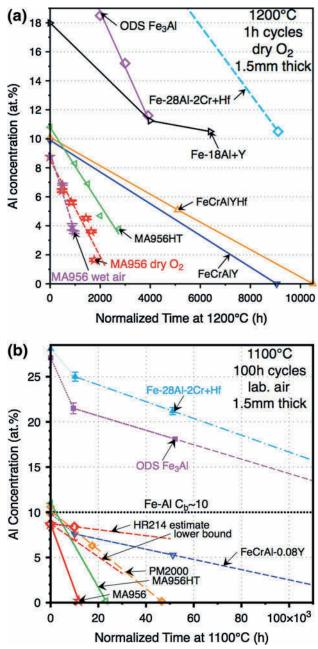
Fig. 3. Change in Al content as a function of normalized exposure time for various alumina-forming alloys (a) in 1-h cycles at 1200°C in dry O<sub>2</sub> and (b) in 100-h cycles at 1100°C in laboratory air. Adapted from Ref. 12.
