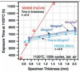
Fig. 1. Time to accelerated attack as a function of specimen thickness for NiCrW alloy 230 and ODS FeCrAI alloy MA956 for exposure in 100-h cycles at 1100°C in laboratory air. For MA956, the time is for the onset of Fe-rich oxide formation and increases significantly with thickness. For 230, the times are to total mass gains of 20–40 mg/cm². Values of *n* are given for Eg. 1. Adapted from Refs. 3 through 5.
