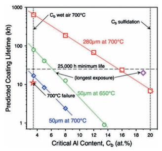
Fig. 4. Predicted coating lifetime as a function of the critical Al content on Gr.91 steels at coating failure for two different coating thicknesses and exposure temperatures. Experimental data points are shown as failure at 700°C (star) and surface coating content at 20 kh (diamond).
