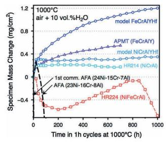
Fig. 7. Specimen mass change during 1-h cycles at  $1000^{\circ}\text{C}$  in wet air (10%  $\text{H}_2\text{O}$ ) for several commercial and experimental alumina-forming alloys.
