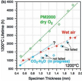
Fig. 6. Time to breakaway as a function of initial specimen thickness comparing dry  $O_2$ , dry air, air with 10%  $H_2O$ , and  $H_2O$ -50%( $CO_2 + 0.15\%O_2$ ) for ODS FeCrAl alloys (a) MA956 and (b) PM2000. In all cases, the specimens are cooled in laboratory air. Adapted from Refs. 5 and 33.
