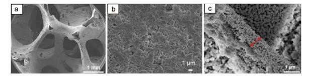
Fig. 12.  $Cr_2O_3$  coatings made with a nitrate concentration of 1.5 M and a plasticizer (PEG 35000) (a) view of the coated foam, (b) view of the homogenous coating, (c) thickness and microstructure of the coating.
