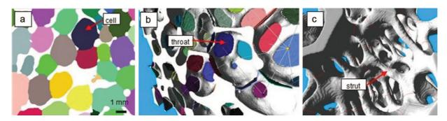
Fig. 5. (a) Segmentation of each cell on a 2D view, (b) segmentation of each throat and connectivity calculation on a 3D view, (c) strut size calculations on a 3D view. (For interpretation of the references to color in the text, the reader is referred to the web version of this article.)
