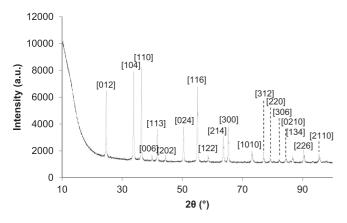
Fig. 10. room temperature XRD pattern of the powder obtained from the calcination sol ( $800 \degree C$  in air) and corresponding to  $Cr_2O_3$  phase.
