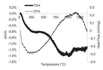
Fig. 14. TG-DT analyzes curves of  $Cr_2O_3$  powder from room temperature to 1400 °C under air (heating rate 300 °C/h).
