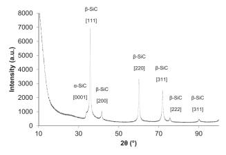
Fig. 1. room temperature XRD pattern of ground β-SiC foam.
