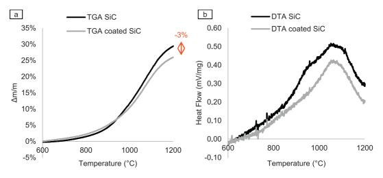
Fig. 13. uncoated and coated SiC after (a) TG and (b) DT analyzes.
