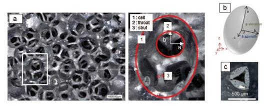
Fig. 3. (a) Optical microscopic image of a foam structure, (b) description of ellipsoid cell parameters, (c) cut of a strut on an optical microscopic image.
