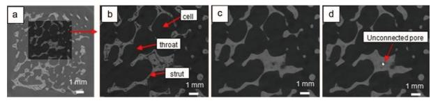
Fig. 4. iMorph 2D reconstruction of a  $\beta$ -SiC foam (a) reconstructed data and choice of a ROI, (b) untreated ROI, (c) after dilatation and erosion, (d) after dilatation and erosion + removal of the unconnected porosity.
