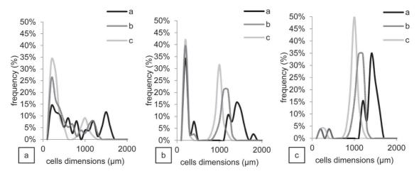
Fig. 6. (a–c) Size distributions of cells (a) with original images, (b) after application of a dilatation-erosion filter, (c) after application of a dilatation-erosion filter and elimination of unconnected porosity.
