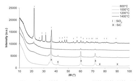
Fig. 9. room temperature XRD pattern of ground SiC foam after heat treatment at 800 °C, 1000 °C, 1200 °C and 1400 °C in air.
