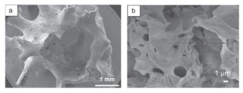
Fig. 11. Cr<sub>2</sub>O<sub>3</sub> coatings made with a nitrate concentration of 1.0 M (a) view of the coated foam, (b) sheet structure of the coating.
