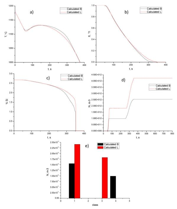
*a* cooling curve; *b* liquid fraction evolution; *c* Si evolution; *d* nodule count evolution; *e* final nodule count 3 1D numerical simulation comparing models B and L
