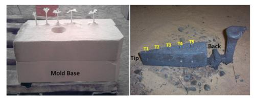
1 Wedge-like casting used in present study showing temperature measurement locations (T1-T5)
