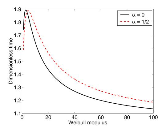
Figure 4: Dimensionless time  $t_{90\%}/t_c$  to reach an obscuration probability equal to 90% as a function of the Weibull modulus m. Two different values of the stress sensitivity exponent  $\alpha$  are considered
