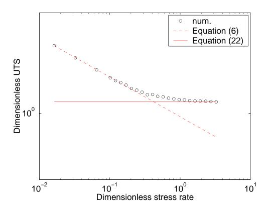
Figure 3: Mean ultimate tensile strength normalized by  $\sigma_c$  as a function of the dimensionless stress rate  $\dot{\sigma}/\dot{\sigma}_c$ . The open circles correspond to the results of 500 Monte Carlo simulations for each considered stress rate (Denoual and Hild, 2000). Two fragmentation regimes are observed. For low stress rates, single fragmentation occurs (Equation (6)) while for high stress rates multiple fragmentations are observed (Equation (22))
