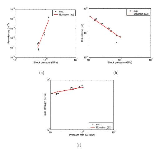
Figure 6: Identification of the two exponents m and  $\alpha$  for tantalum. (a): Pore density vs. shock pressure. (b): Critical time vs. stress rate. (c): Spall strength vs. stress rate. The open circles are experimental data (Roy, 2003), and the solid lines are results given by Equation (32) when m=8 and  $\alpha=4.5$
