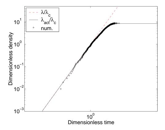
Figure 1: Dimensionless densities as functions of dimensionless time  $t/t_c$  for the ring expansion simulation. The dashed line corresponds to the intensity of the Poisson point process, the solid line is the closed-form solution (19) when m=10 and  $\alpha=0$ . The crosses are the results of a Monte Carlo simulation ( $\lambda_c L=100$  and  $\lambda_c \delta=10^{-3}$ )
