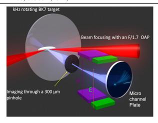
FIG. 1 (color online). Scheme of the experimental setup.
