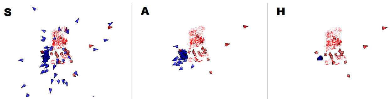
Fig. 11. Desk dataset : 100 poses computed with N = 5,000 RANSAC iterations. In H , the standard deviation is 3.04% of the distance to the scene.
