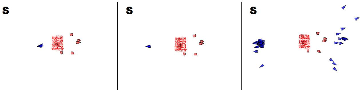
Fig. 13. Wall dataset : 100 pose computations with  $N = 300$  RANSAC iterations for the three test views (see 12) in scenario **S**. From left to right: Test views 1 to 3. The standard deviation is 2.14% of the distance to the scene in view 1 and 0.12% in view 2.
